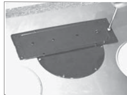
5. Mount rectangular plate (previously removed) on top of transition adapter.
